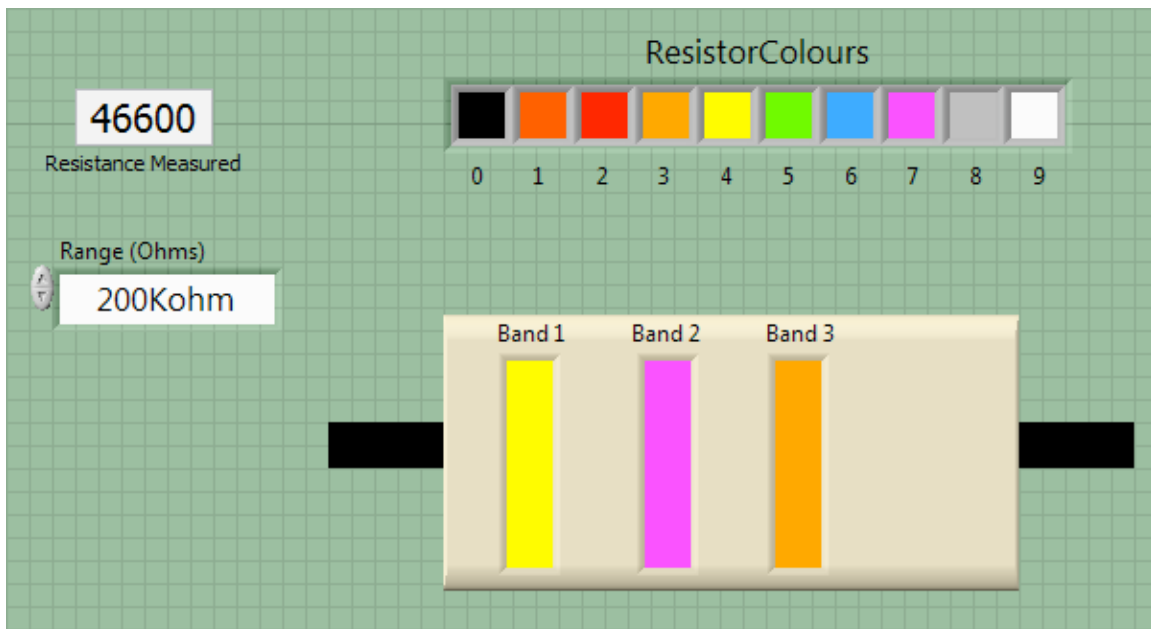
Fig. 6 Measurement and Colors of a Nominal 47 kW Resistor
